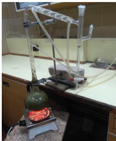
Figure 3. Essential oil isolation by Clevenger apparatus.
