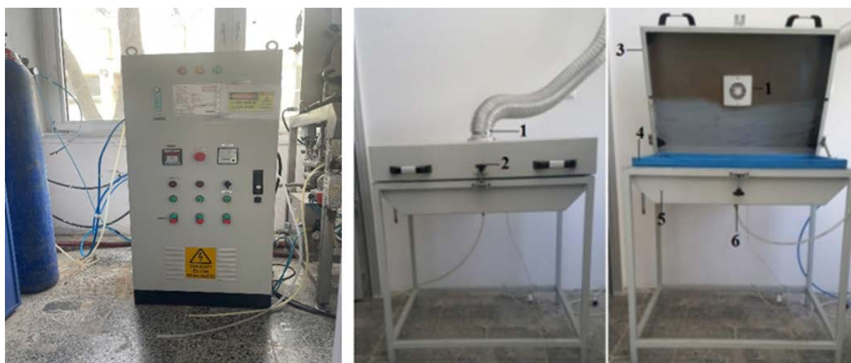
Figure 2. Ozone generator and printing device (1. Ozone Discharge Fan, 2. Screw, 3. Top Cover, 4. Templates, 5. Conical Subtank, 6. Ozone Supply Inlet) [36]
