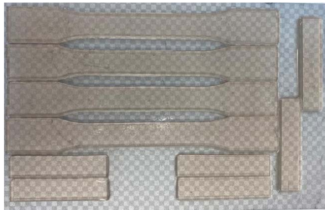
Figure 2. Layout of nanocomposite specimens on the printing bed.
