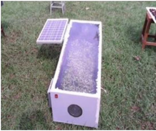
Figure 1. A direct active solar dryers ( Alonge and Uduak, 2014 ).
