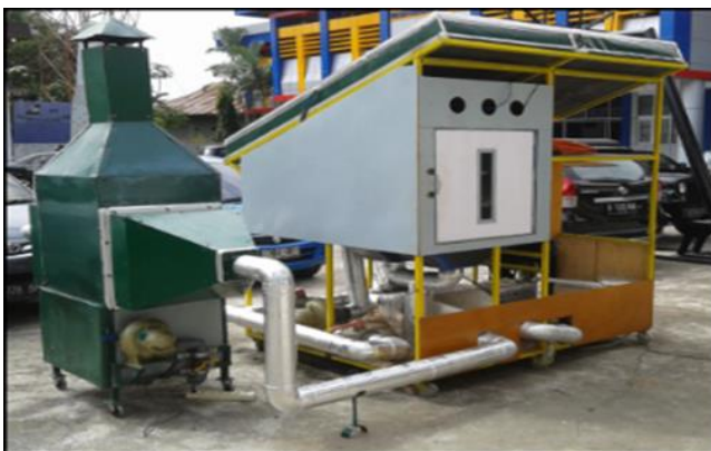
Figure 5. Solar assisted heat pump dryer integrated with biomass furnace ( Yahya, 2016 ).
