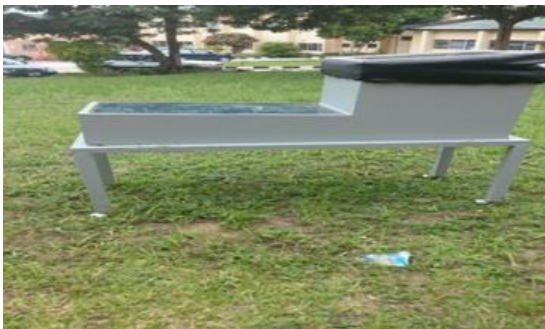
Figure 3. Mixed mode solar dryer ( Alonge et al., 2020 ).
