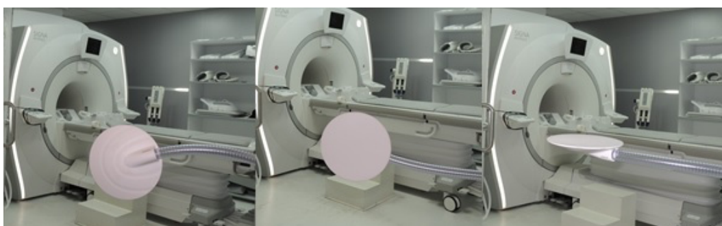
Fig. 3. The apparatus called "passive driver," which is one of the extra equipment for MRE examination, is shown from the back, front, and side in three images from left to right.
