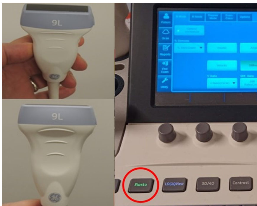
Fig. 1. Touch panel and button panel of GE Logic S8 brand/model USG device with elastography software (elastography button is circled in red on the right) and a 9 Mhz linear probe with hardware elastography features (shown from two different directions on the left).
