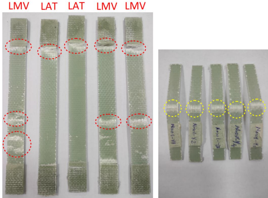
Figure 10. Damage mechanism of tensile and flexural test samples
