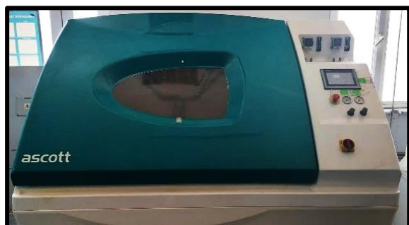
Figure 7. Cabinets for salt spray test (a) and cycle tests (b)
