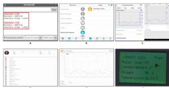
Figure 24. GSR results: (a) in serial monitor; (b) in mobile application; (c) waves in the mobile application; (d) in web server; (e) waves in web server; (f) in GLCD
