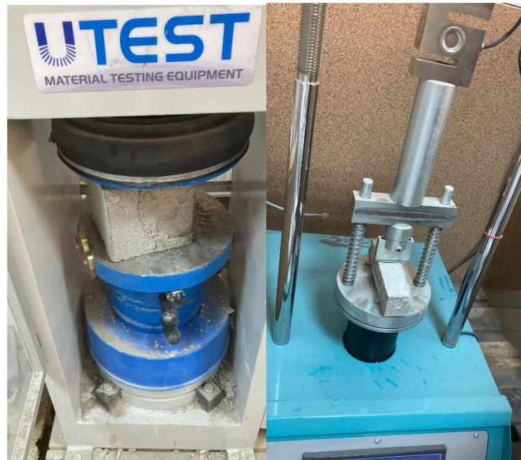
Figure 2. Compression and flexural test
