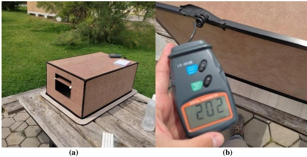
**Figure 5.** (a): Daylight measurement with the physical model. (b): The value obtained from the luxmeter.
