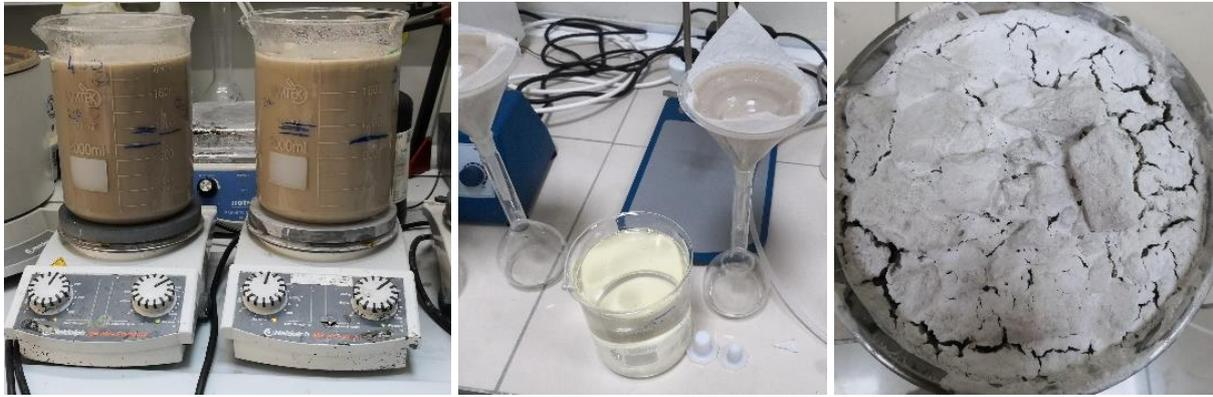
**Figure 2.** Leaching process (left image), filter and leaching liquid (medium image), and the resulting filter cake (right image)
