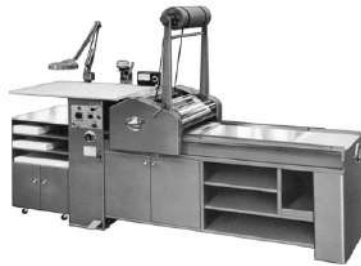
Figure 6. VANDERCOOK Universal III 18 3 / 4 ” × 28-inch (47,62 x 71,12 cm) letterpress proof machine, 1959, USA (Vandercookpress, 2023).
