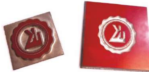
Figure 3. Cliché examples for printing, hot foiling, (left) and embossing (right), Ankara. (Researcher's archive, 2023).
