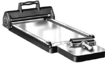
Figure 5. VANDERCOOK NO. 0 12 3 / 4 × 27-inch (32,38 x 68,58cm) letterpress proof press, 1950, USA (Letterpresscommons, 2023).
