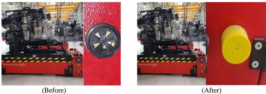
Figure 2. Elimination of noise fans of AGVs
