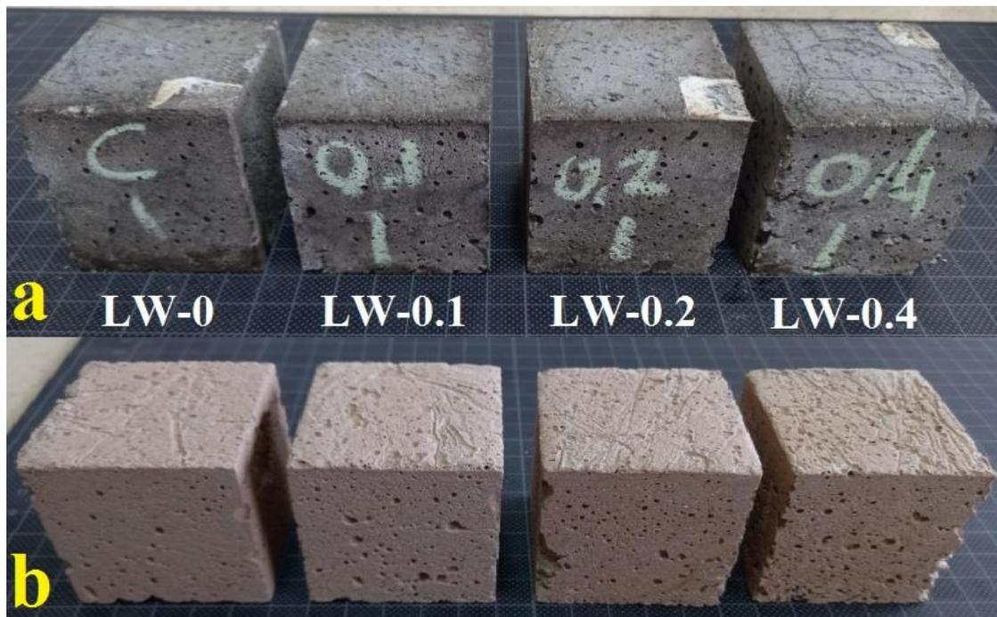
**Figure 6.** Pictures of specimens (a: before high-temperature test, b: after high temperature test)
