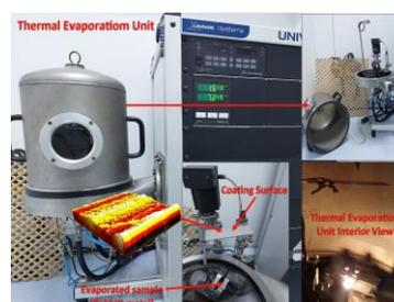
**Figure 1.** Detailed View of the Device of the Thermal Evaporation System
