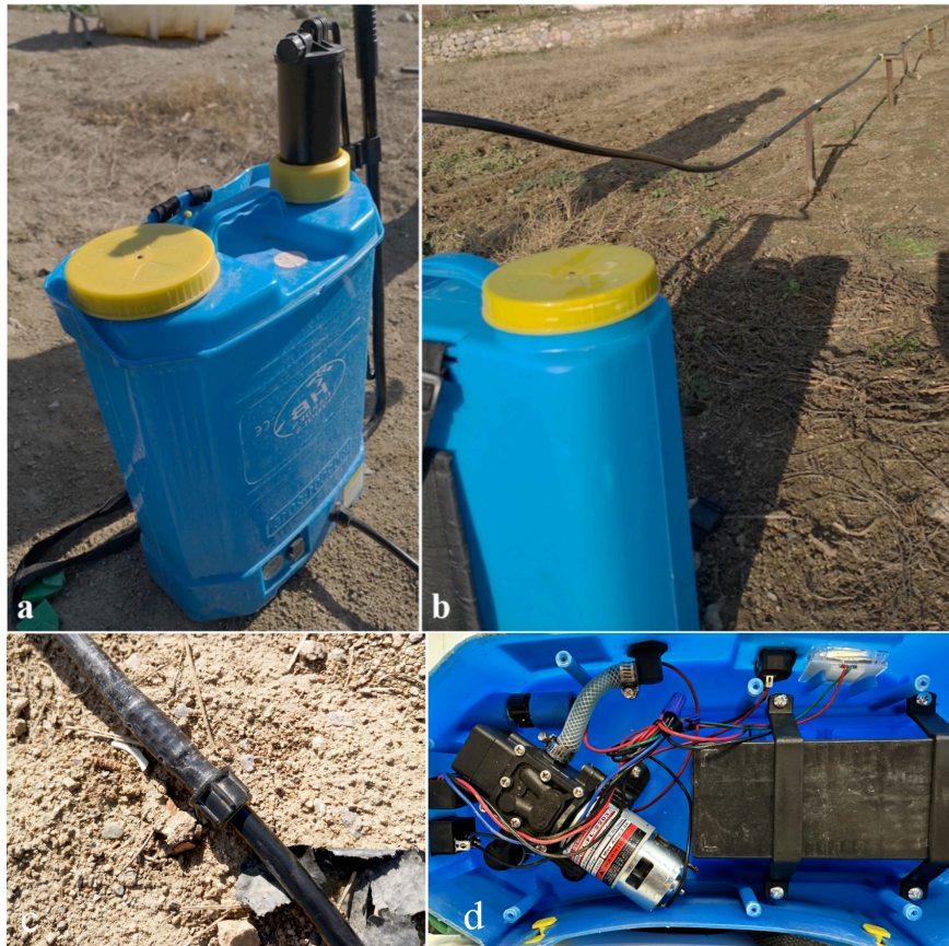
Figure 1. Modular application method. Battery-powered backpack sprayer was combined with different types of driplines. Main body (a), coupled with the dripline (b), coupling part (c) and battery (d).
