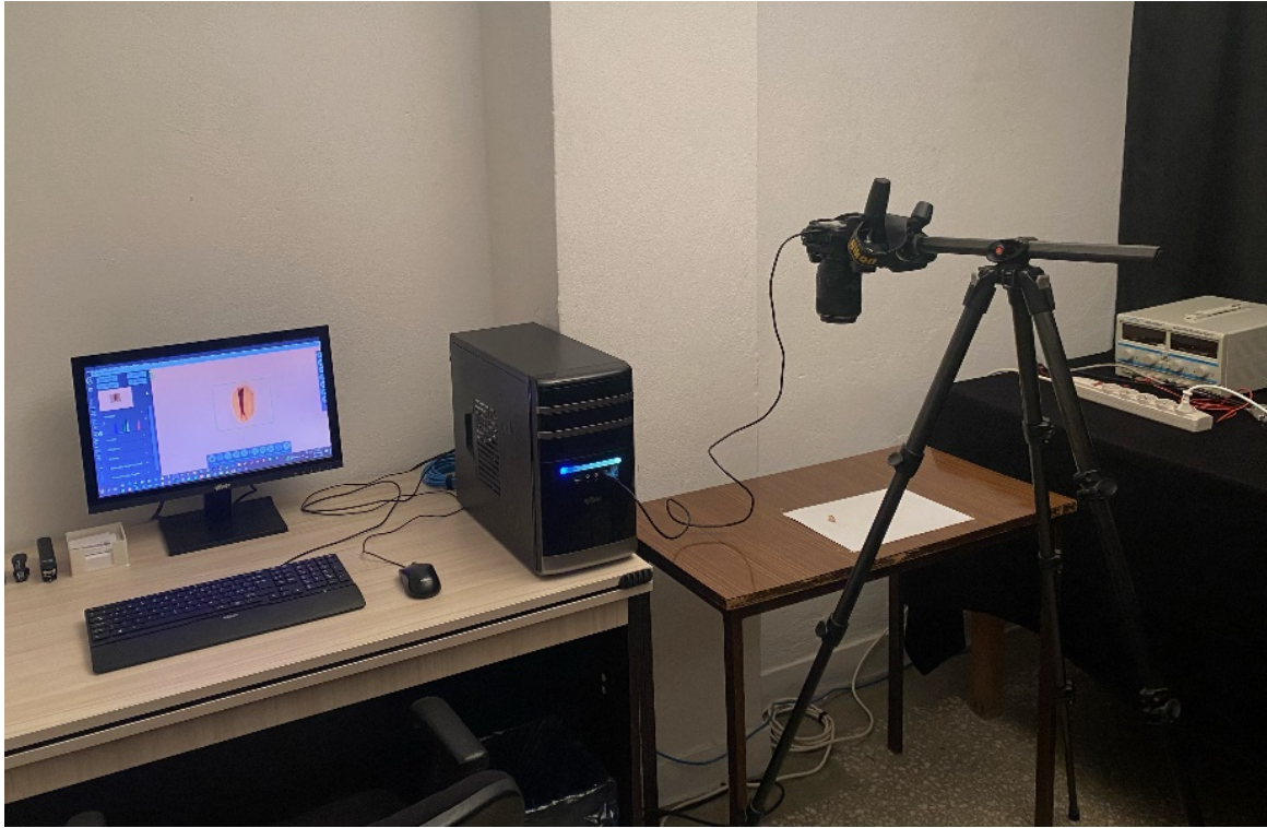
Figure 2. Antep pistachio nuts image capture set-up.
