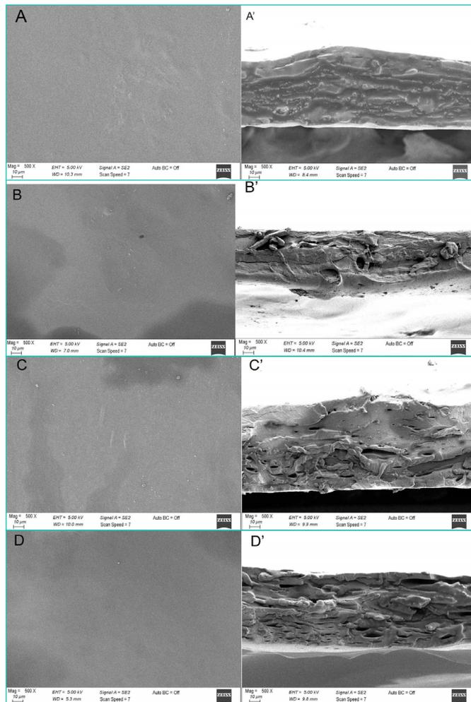
**Figure 2.** SEM images of surface (A, B, C, and D) and cross-section (A', B', C', and D') of the control film and films containing 2%, 4% and 6% of NSNE, respectively
