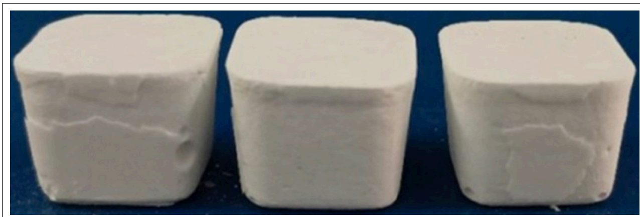
Figure 4. Magnesium phosphate cement specimen.
