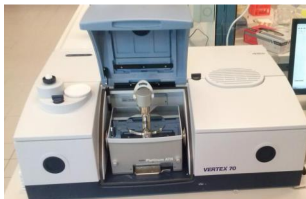
Figure 1. FTIR Spectroscopy Device
