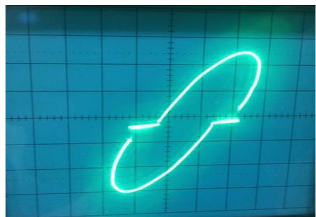
Figure 9. The graph of the variation of the discharge voltage of the Sphere-Plane electrode system at 50 Hz versus the discharge current
