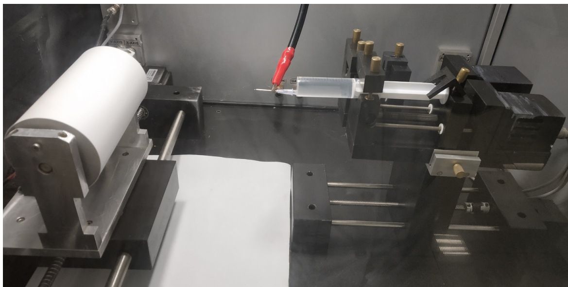
Figure 1. Electrospinning setup (E-SPIN NANO) for fabrication of MUP-PCL-TEO-PVA bilayer nanofiber scaffold.
