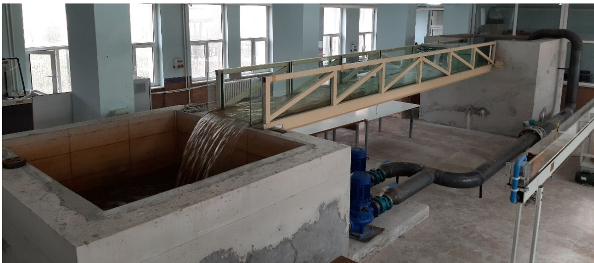
Figure 5. Open channel system
