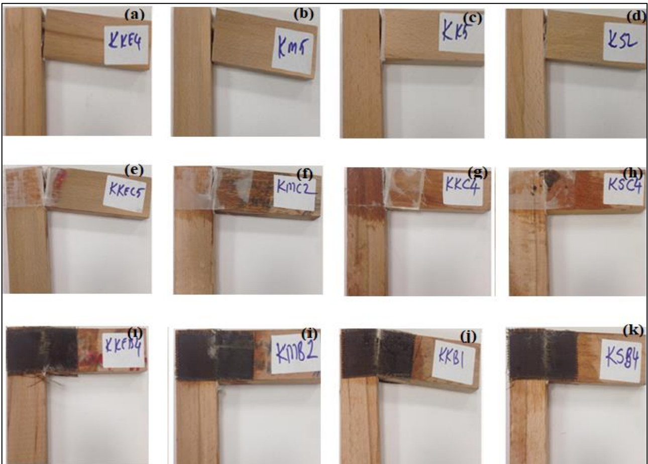
Figure 4. Failure modes of the experimental samples under bending strength test. (a) Chestnut dowel joints. (b) Oak dowel joints. (c) Beech dowel joints. (d) Scots pine dowel joints. (e) Chestnut dowel + GFRPWF joints. (f) Oak dowel + GFRPWF joints. (g) Beech dowel + GFRPWF joints. (h) Scots pine dowel + GFRPWF joints. (i) Chestnut dowel + BFRPWF joints. (j) Oak dowel + BFRPWF joints. (k) Scots pine dowel + BFRPWF joints.
