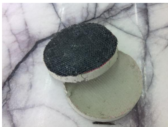
Figure 1. Consolidation test samples placed with geotextile (Dikmen, 2013)
