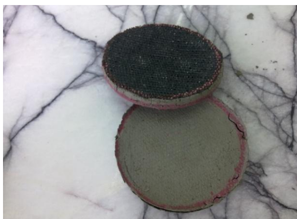
Figure 1. Consolidation test samples placed with geotextile (Dikmen, 2013)
