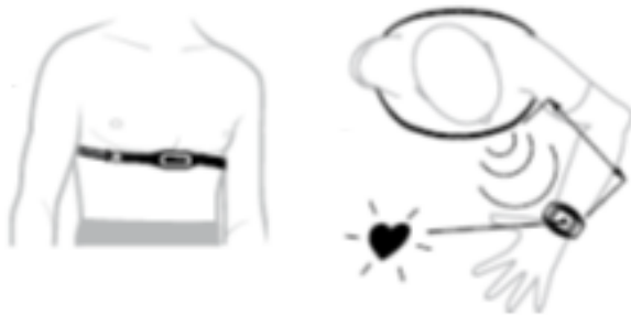
Figure 2. Attachment method of the chest band.
