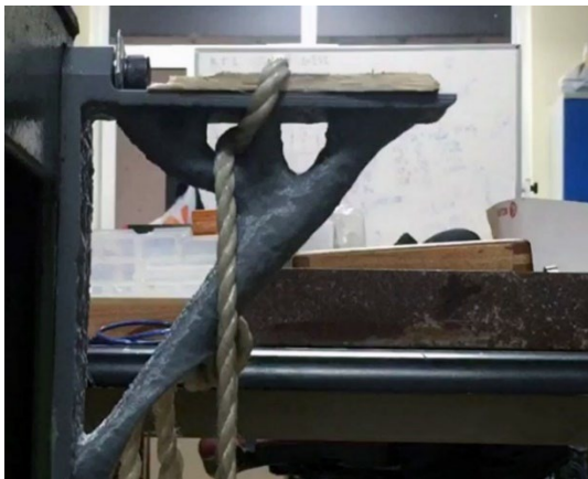
Figure 9. The connecting mechanism of the 155-135 mm bracket.
