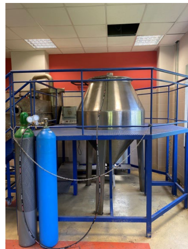
Figure 1. Gas atomization system used during experimental studies.
