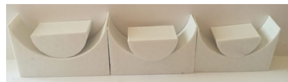
Figure 4. 3D printed bending test apparatus.
