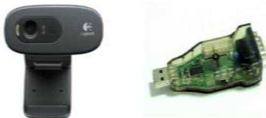
Figure 1. USB camera and USB2Dynamixel control card.
