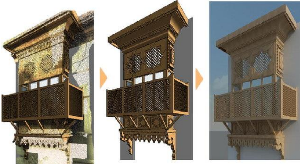
Figure 2. Transferring a historical bay window, from point cloud to 3D Model, then to BIM [25]
