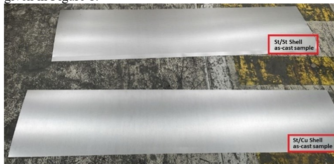
Figure 1. As-cast samples produced via steel/steel and steel/copper shell pair
