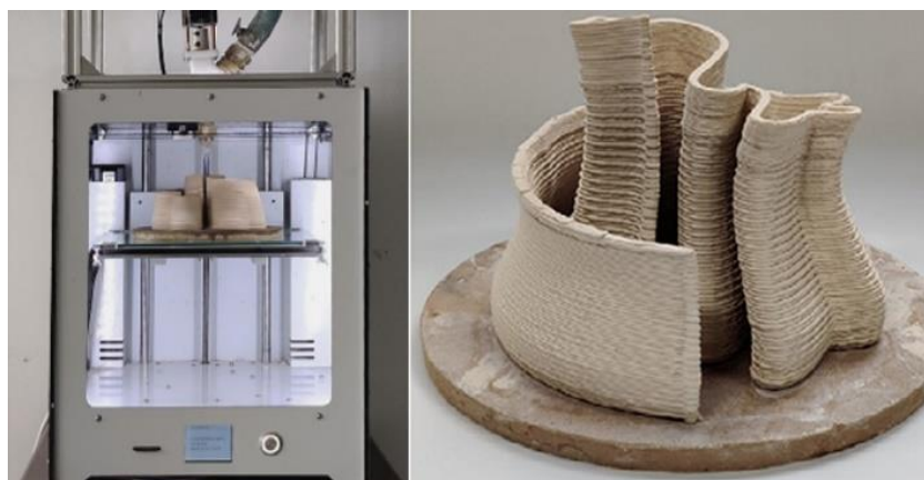
Figure 21: A 3d ceramic printer in operation and the resulting ceramic product, (Zhong et al., 2020, pp. 113-114).
