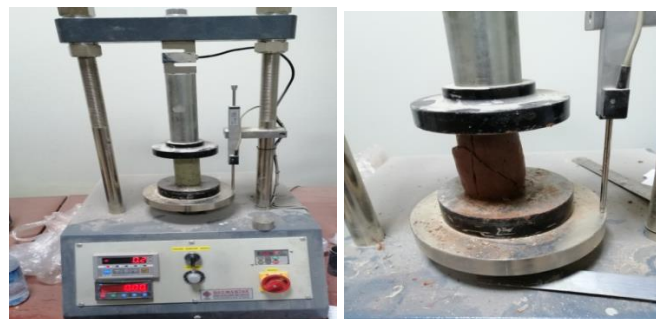
Figure 6. UCS machine and failed samples
