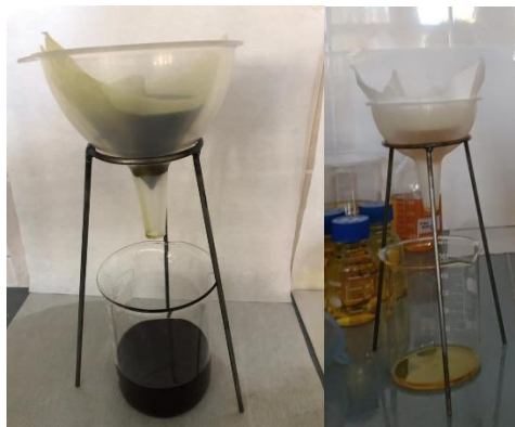
Figure 3. Filtration process applied to waste pumpkin seed and camelina oils
