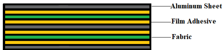
Figure 4. Al sheets, hybrid fabrics and adhesives sequences
