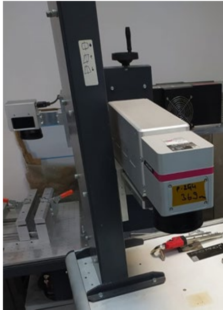
Figure 1. Laser marking machine-100 W
