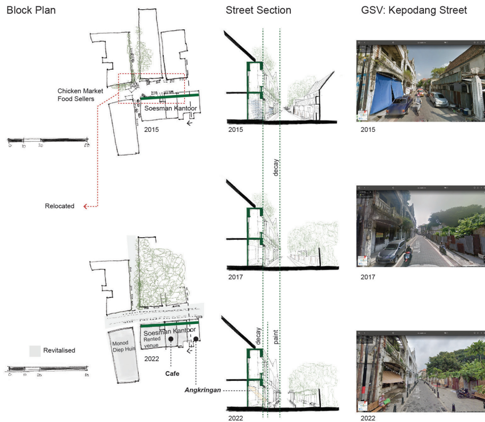
Figure 7. Diagram of changes around Soesman Kantor before, during and after revitalisation (Author in reference to GSV of Kepodang Street (timestamps: 2015, 2017, 2022), 2024)
