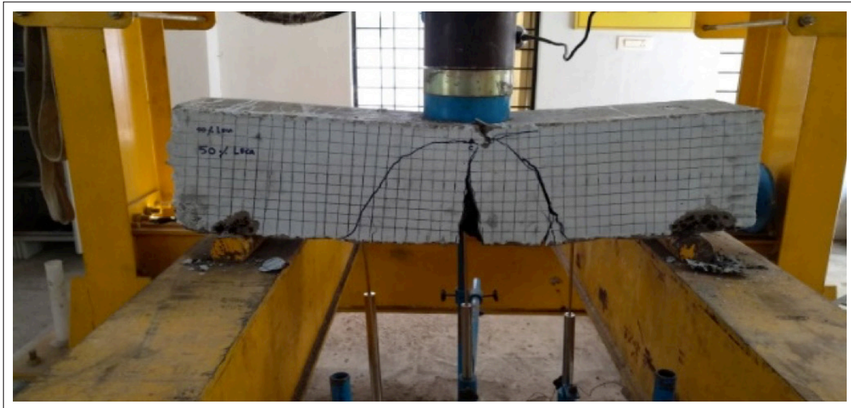
Figure 12. Crack pattern of beam LECA 25.
