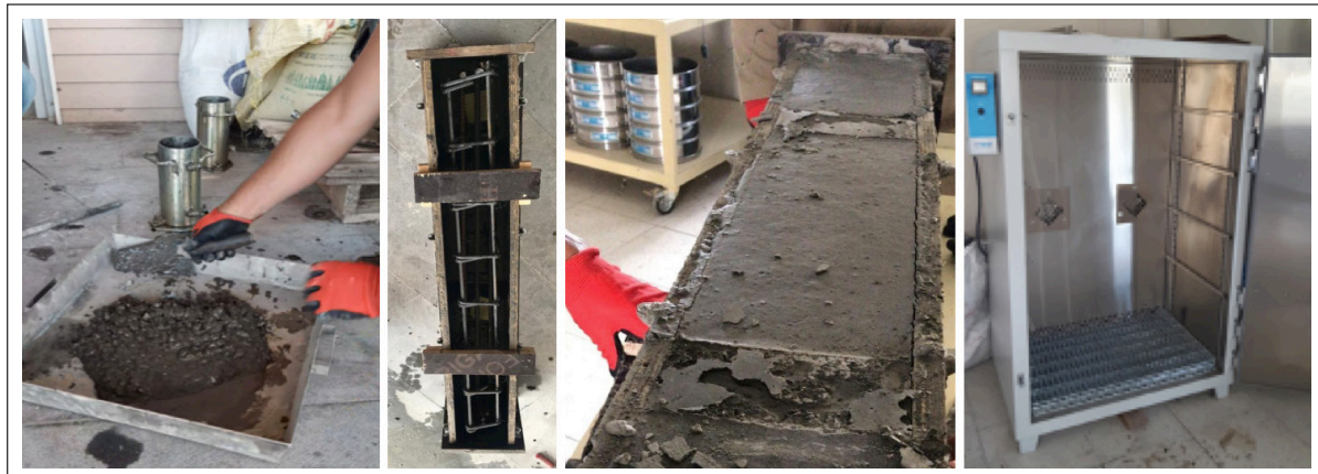
Figure 2. Placing and curing concrete in molds.
