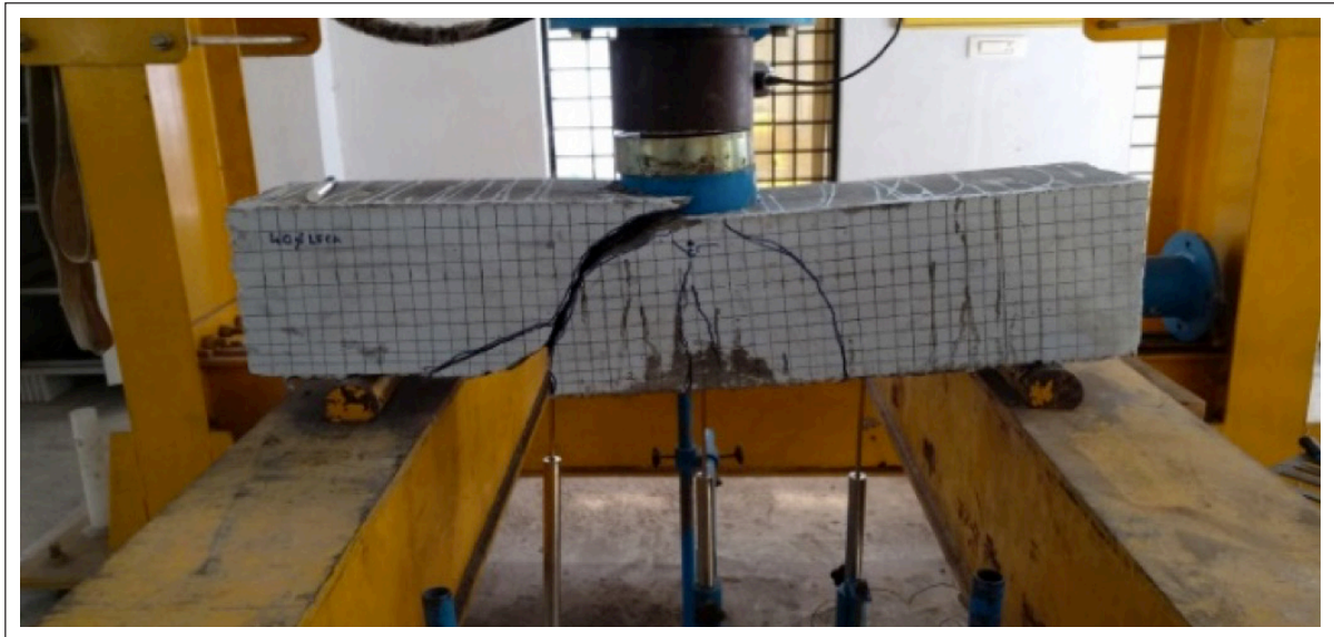
Figure 11. Crack pattern of beam LECA 20.
