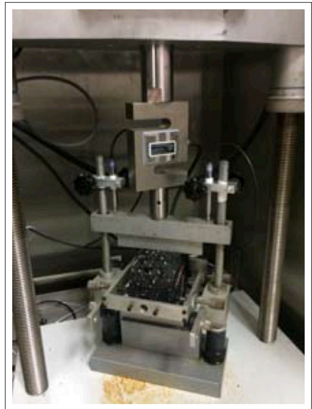
Figure 7. Indirect tensile fatigue test.
