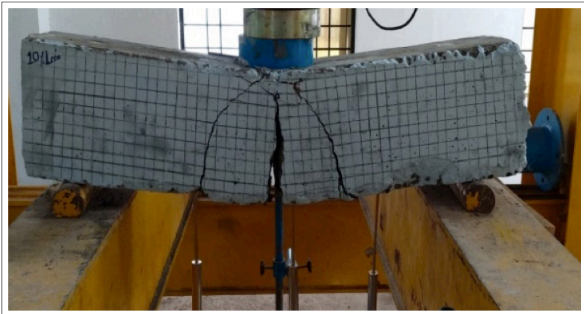
Figure 8. Crack pattern of beam LECA 5.
