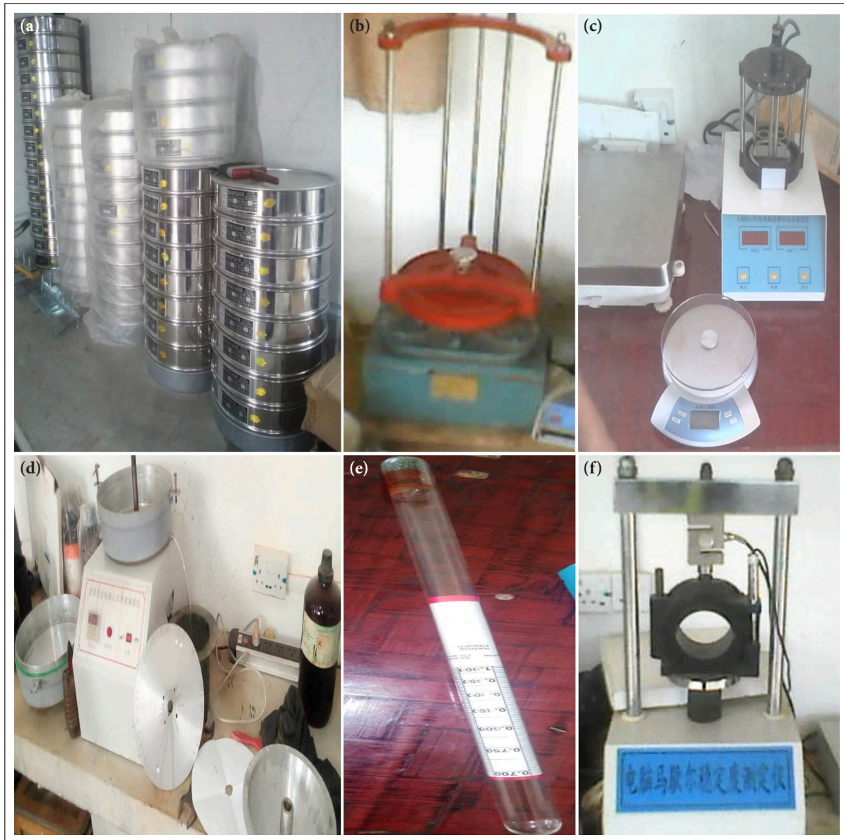
Figure 1. (a) Set of Sieves (b) Sieve Shaking Machine (c) Weighing Balances (d) Bitumen Extraction Machine (e) Thermometer (f) Marshall Testing Machine.
