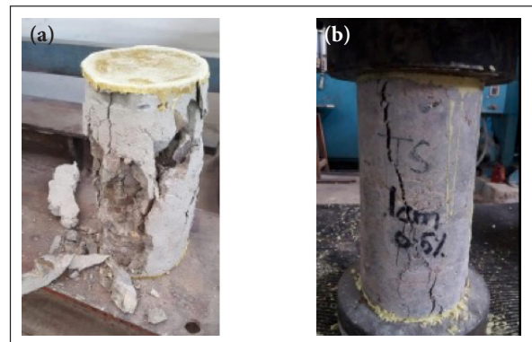
Figure 7. Typical failure pattern exhibited by (a) plain concrete and (b) JFRC specimens under uniaxial compression.
