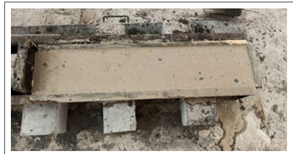
Figure 2. Mould with casted beam specimen.
