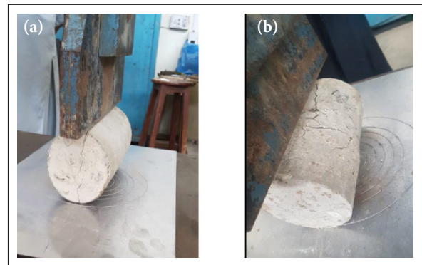
Figure 9. A typical failure pattern is exhibited by (a) plain concrete and (b) JFRC specimens under tensile splitting.
