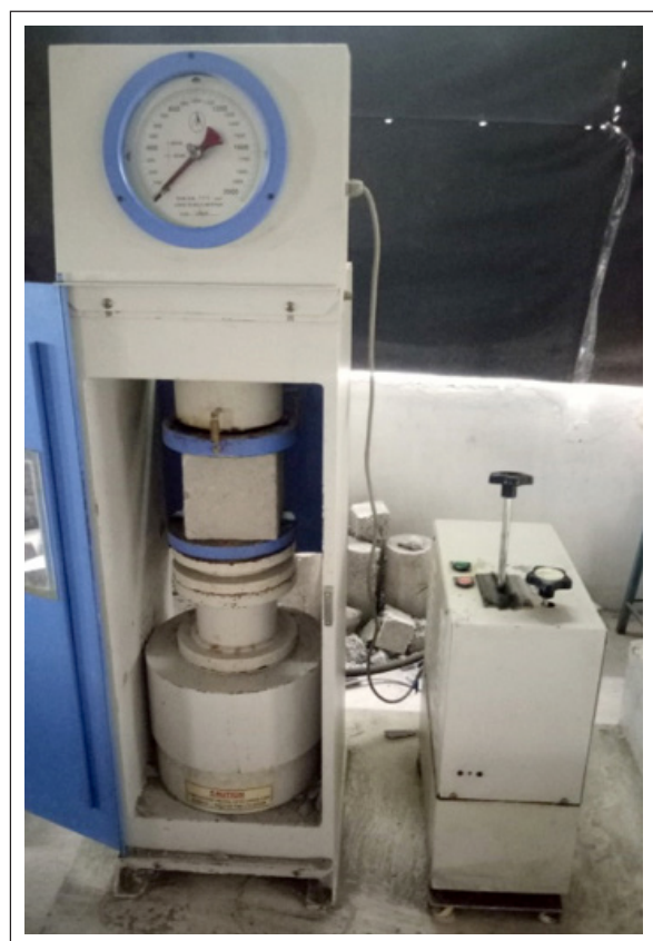
Figure 5. Experimental photograph of compressive strength test.
