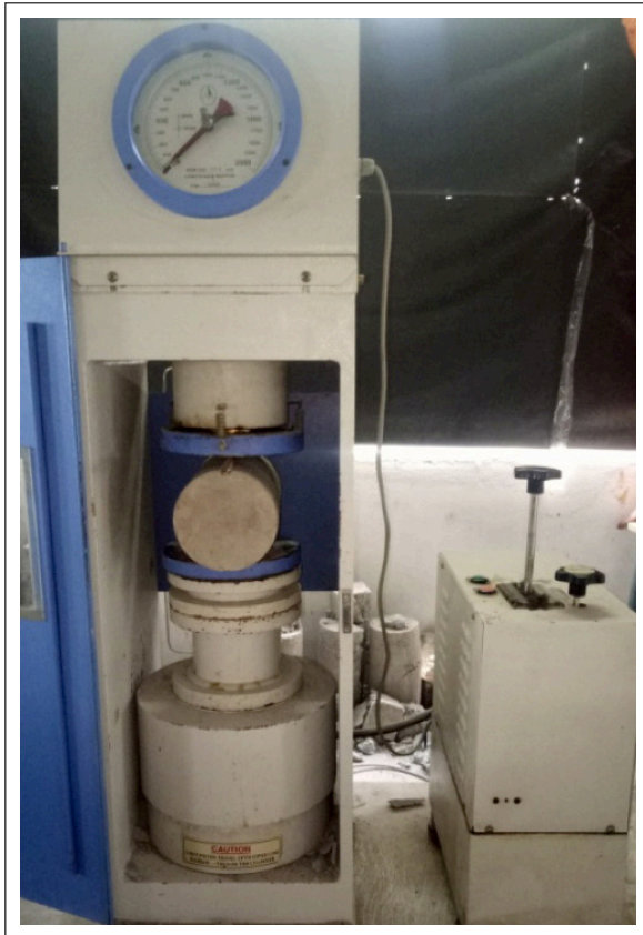
Figure 6. Experimental photograph of Split tensile strength test.
