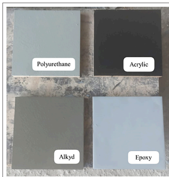
Figure 1. Polyurethane, acrylic, alkyd, and epoxy coated panels.
