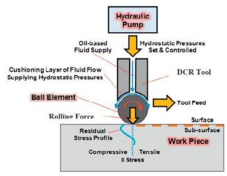
Figure 3. Working principles of deep rolling process
