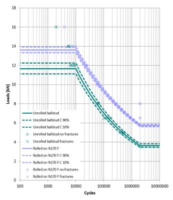
Figure 8. F-N curve comparison of ball stud in rolled at %170 F and un-rolled condition.
