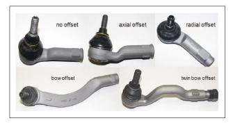
Figure 2. Outer tie rod housing variations [6]
