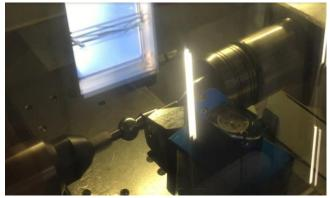
Figure 5. Application of deep rolling process
