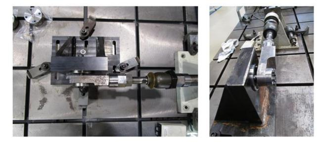
Figure 6. Experimental set-up of ball stud fatigue test
