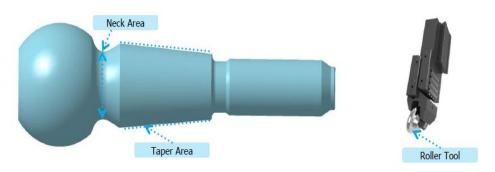
Figure 4. Schematic representation of the ball stud and roller tool
