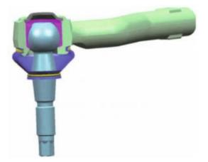
Figure 1. Outer tie rod assembly [6]
