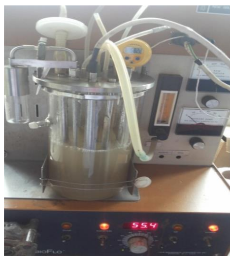
Figure 7. New Brunswick Scientific BioFlow C-32 fermenter (1.5 L) showing the reaction containing resting cells of APB-6 for the biotransformation of butyramide to butyrohoxamic acid.
