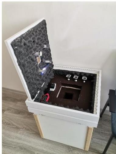
**Figure 2.** Specially Prepared Insulated Sound Transmission Measurement Box
