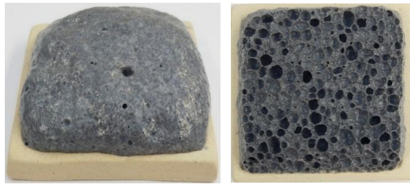
Figure 9. a) Blistering image of 7% SiC added glaze b) Crater image revealed by engraving the top surface of 7% SiC added glaze.
