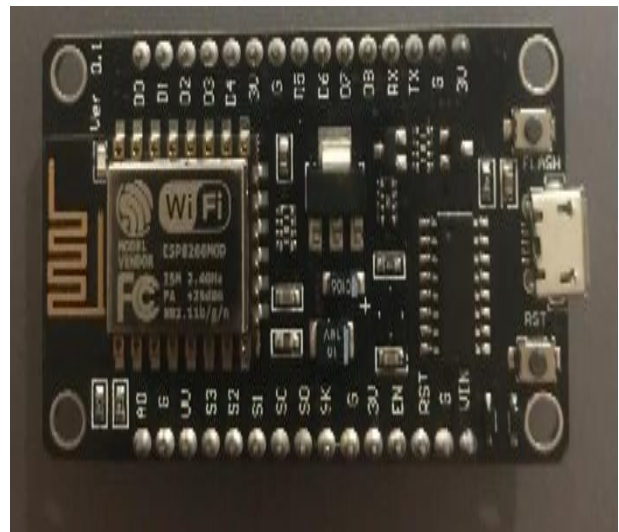
Figure 1. NodeMCU with ESP8266 Wi-Fi module
