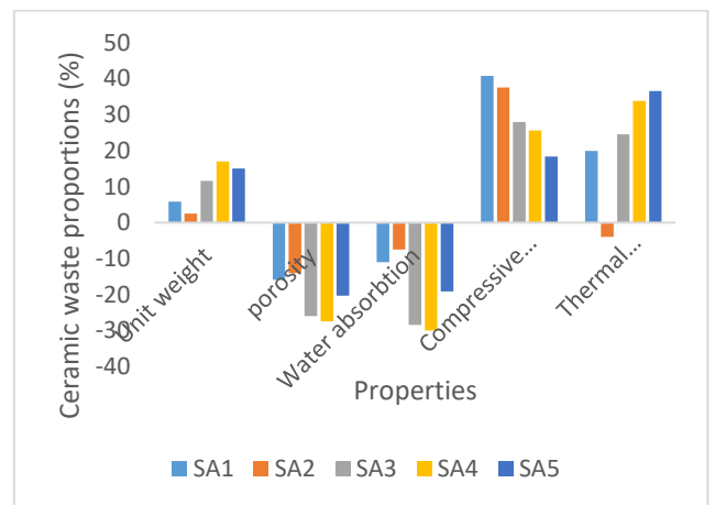
Figure 16. Percentage change of ceramic waste according to properties
