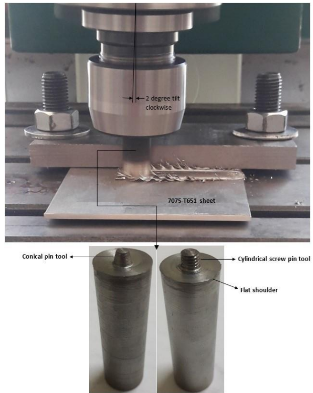
Figure 2. FSLW of alloys and the used welding tools
