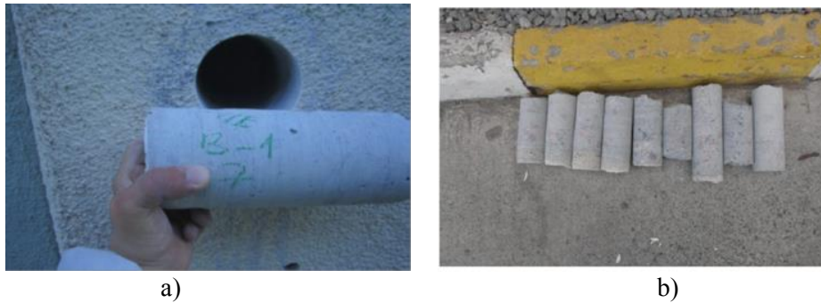
Figure 4. a) b) Concrete core sampling
