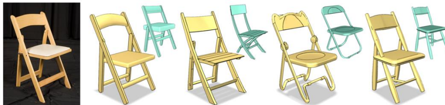
Figure 2: 3D modelling of a chair inspired by four different 3D options (cyan) from a photograph. New models (yellow) are created as geometric variations of the candidates to match the target product in the photo while maintaining the 3D structure of the options [61].
