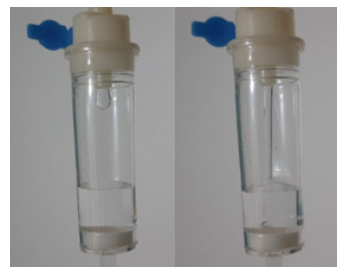
Figure 2 A) Flow in Drop Form, B) Flow in Continuous Form
