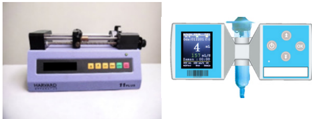
Figure 5 A) Syringe Pump B) Placement of the Measuring Device in the Drop Chamber
