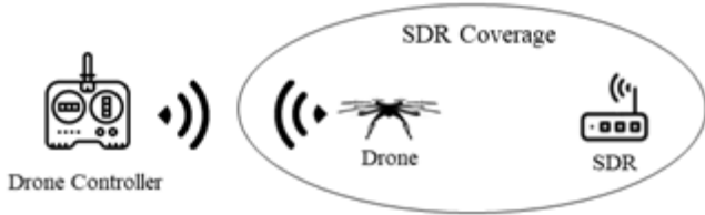
Figure 6. The SDR coverage in our simulation system shows that drone controllers are always out of coverage.
