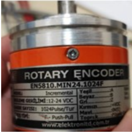
FIGURE 1. (a). Used rotary encoder, (b) Output pulses and period relation for A, B and Z channels respectively.
