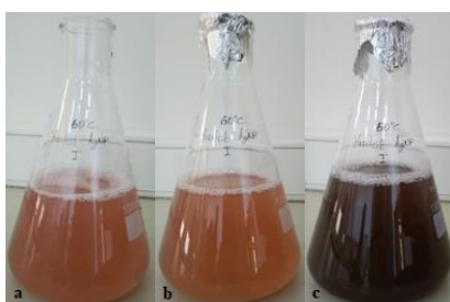
Figure 4- AgNP solution obtained from cornelian cherry extract prepared at 60 °C (a) 0 min, (b) 90 min, (c) 24 hours
