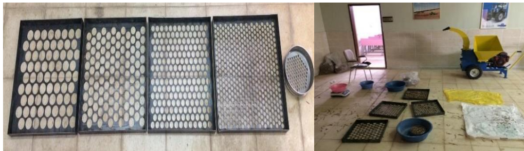
Figure 2. Sieves in different hole diameters used in the study and sieving
