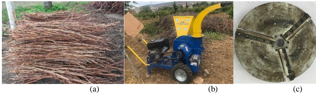
Figure 1. Pruning branches and shredding machine and chopper blade
