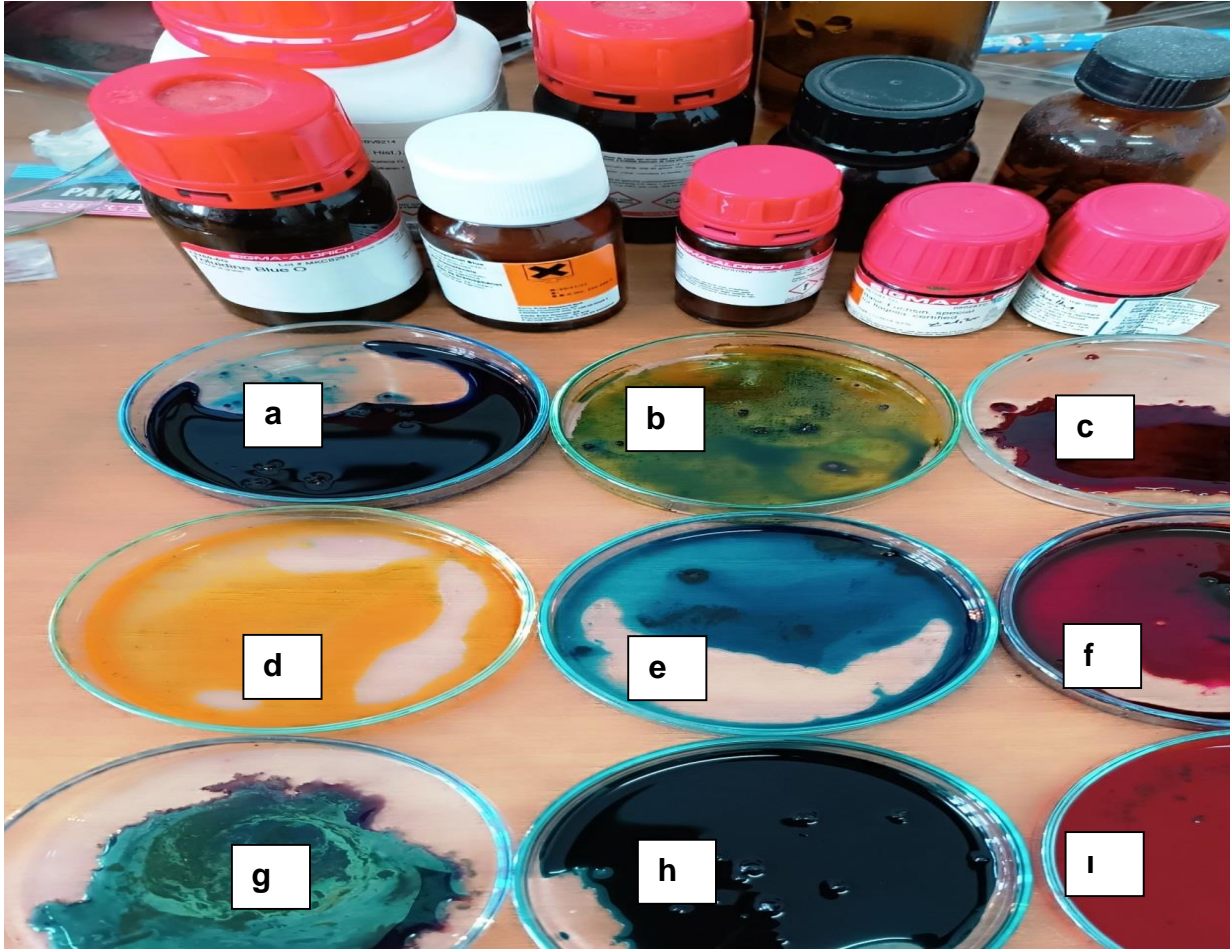
Şekil 1. Araştırmada kullanılan boyama maddeleri a) Toluidine blue O, b) Aniline blue, c) Safranin O, d) Bromophenol blue, e)Methyl green, f) Basic fuchsin, g) Giemsa stain, h) Fast green FCF, i) Carmin. Figure 1. Staining substances used in the research a) Toluidine blue O, b) Aniline blue, c) Safranin O, d) Bromophenol blue, e)Methyl green, f) Basic fuchsin, g) Giemsa stain, h) Fast green FCF, i) Carmin.
