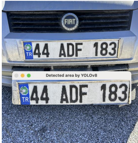
Fig. 6. Example of plate region detected with YOLOv8 model.
