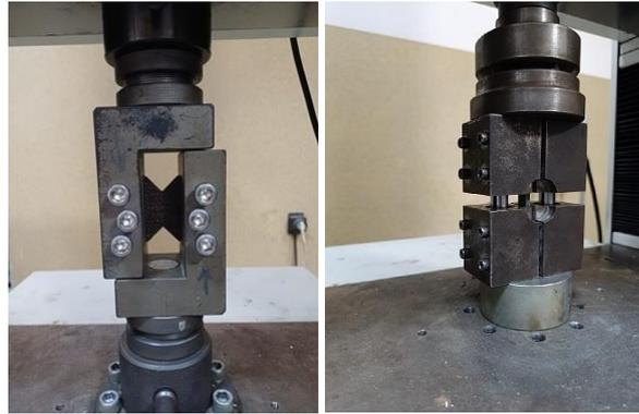
Figure 9. Shear and Compression Test Apparatus
