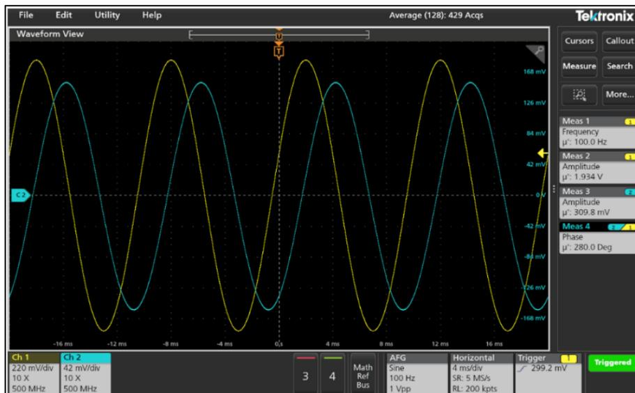
Figure 7. Waveforms of the proposed active floating inductance simulator that are being tested for voltage & current.
