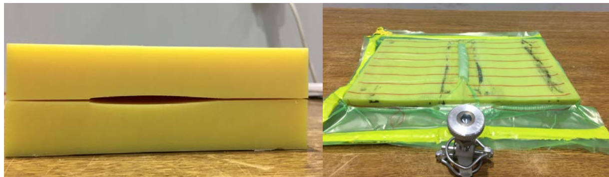
Figure 1. Mold system and vacuum infusion process of the wings
