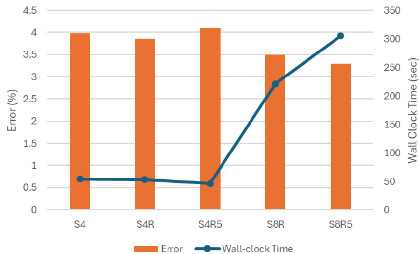
Figure 9. Error and analysis time comparison of element types for critical local elastic buckling load of RHS under minor axis bending
