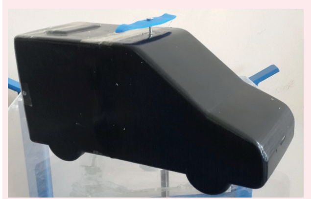
Figure 5. Test model 1 and front spoiler application
