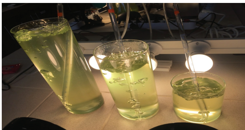
Figure 1. The photobioreactors with different height/diameter ratio.
