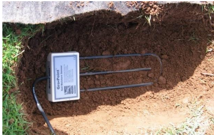
Figure 4. An image of a time-space transmissometer device (Soil Sensor, 2021b).
