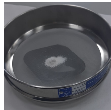
Figure 3. Enamel powder standardized by sieve
