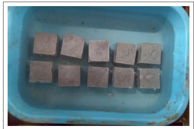
Figure 5. Water absorption test setup.
