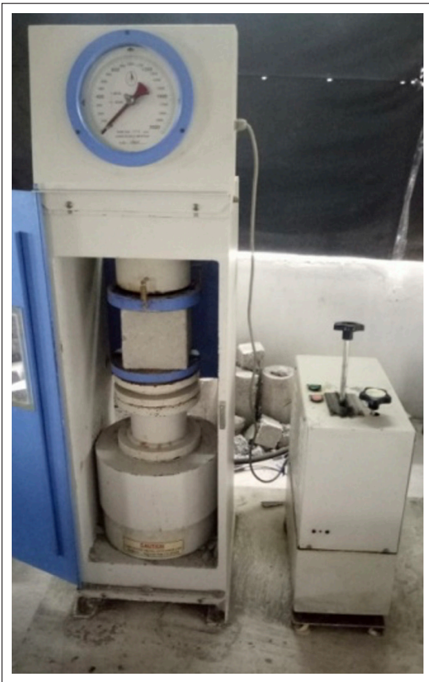
Figure 3. Compressive strength setup.
